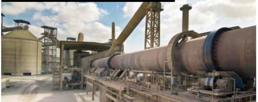
On a per capita basis, the consumption of cement is second only to water and there are currently no substitutions. Therefore, it is critical that neither product quality nor productivity is impinged. For these reasons, oxygen-enhanced combustion in cement kilns is a proven solution to provide the GHG emissions reductions needed over the next 10-15 years before long-term solutions are sufficiently deployed.
