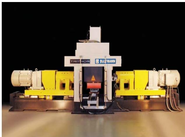
Superconducting induction billet heater
