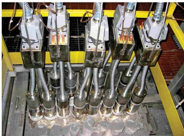
Immersion heating system using array of 15 heaters at a net 97% energy efficiency
