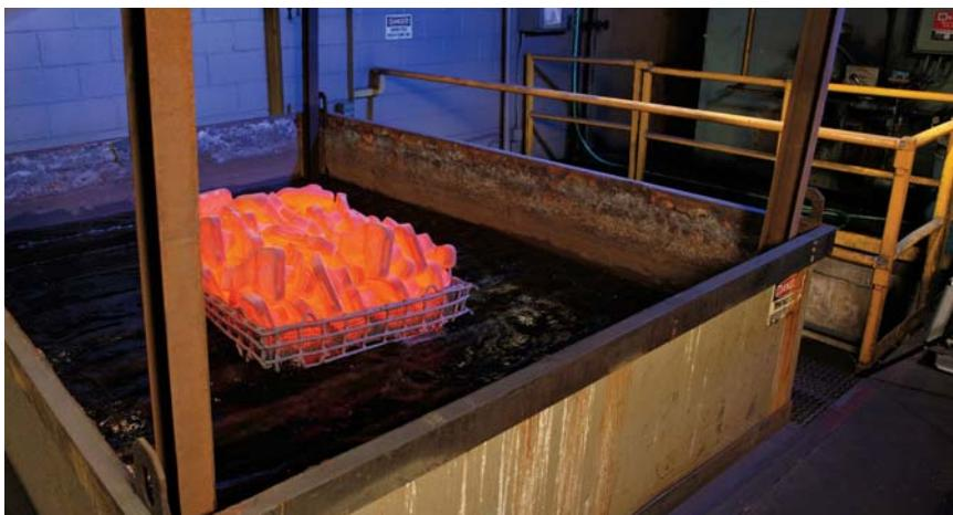
Load of parts being quenched in polymer-based quenchant
