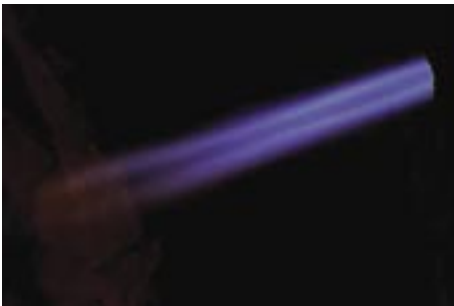
Shrouded supersonic lance Decarburisation, energy introduction and bath agitation.
