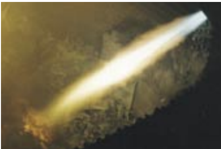
Soft Lance Scrap cutting with rigid oxygen stream. Post combustion with soft oxygen.
